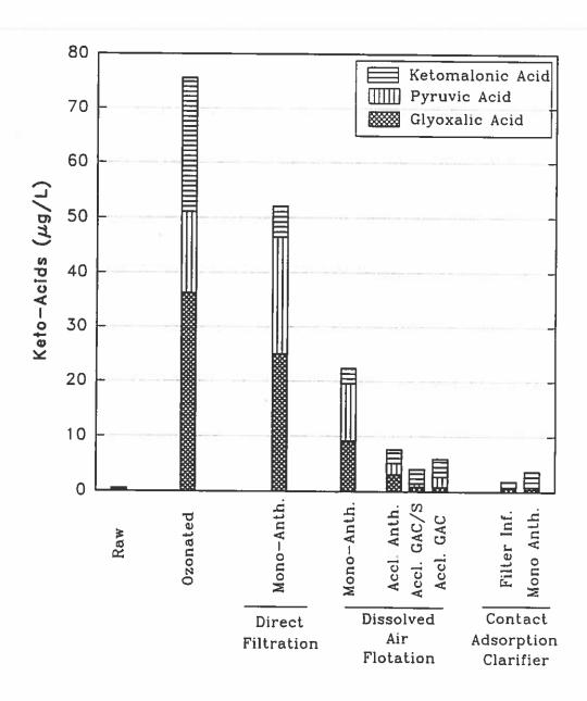
Figure 12. Keto-acid Concentrations at Various Stages of Treatment on May 14, 1992. (All are filter effluents unless otherwise indicated; Accl=acclimated; GAC/S=dual media filter with F300 and sand; GAC=mono-media filter with Nuchar B)
