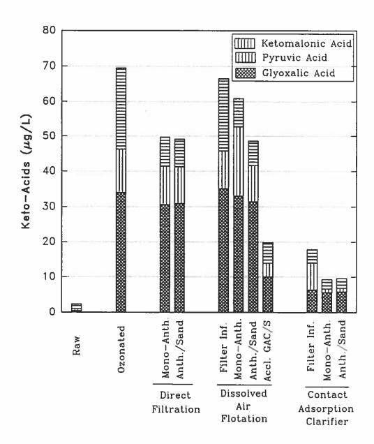
Figure 13. Keto-acid Concentrations at Various Stages of Treatment on February 6, 1992. (All are filter effluents unless otherwise indicated; Accl. GAC/S=acclimated dual-media filter with F300 and sand
