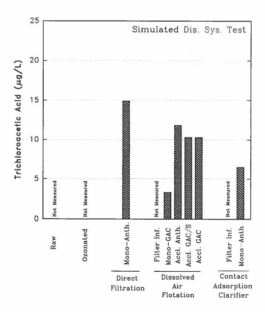
Figure 7. Trichloroacetic Acid Formation from the Simulated Distribution System Test in the Pilot Filter Effluents on August 4, 1992. (All are filter effluents unless otherwise indicated; Mono-GAC=fresh mono-media GAC filter with F300; Accl. Anth. =acclimated mono-media anthracite filter; Accl. GAC/S=acclimated GAC/Sand dual-media with F300; Accl. GAC=acclimated GAC mono-media filter with Nuchar B)
