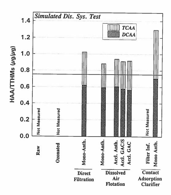
Figure 15. Haloacid to Trihalomethane Simulated Distribution System Test Ratios at Various Stages of Treatment on May 14, 1992. (All are filter effluents unless otherwise indicated; Accl=acclimated; GAC/S=dual media filter with F300 and sand; GAC=mono-media filter with Nuchar B)
