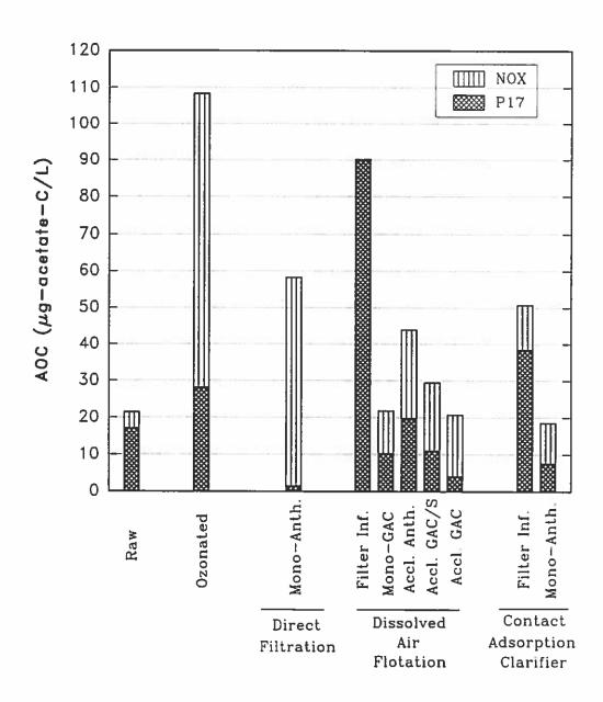
Figure 2. Assimilable Organic Carbon Concentrations at Various Stages of Treatment on August 4, 1992. (All are filter effluents unless otherwise indicated; Mono-GAC=fresh mono-media GAC filter with F300; Accl. Anth. =acclimated mono-media anthracite filter; Accl. GAC/S=acclimated GAC/Sand dual-media with F300; Accl. GAC=acclimated GAC mono-media filter with Nuchar B)
