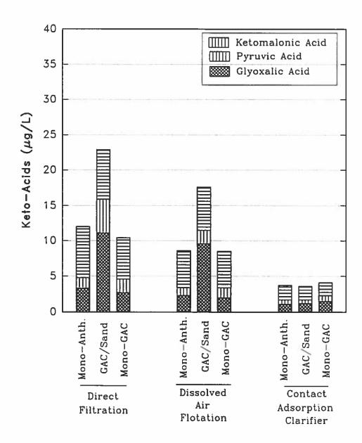
Figure 9. Keto-acid Concentrations in the Effluents of the Three Acclimated Filters for the Period February 17-20, 1992. (Mono-Anth.=mono-media anthracite filter; GAC/Sand=dual-media filter with F300 and sand; Mono-GAC=mono-media filter with Nuchar B)
