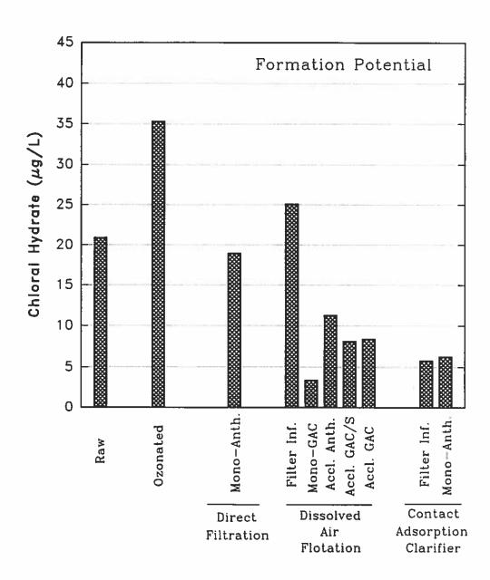
Figure 8. Chloral Hydrate Formation Potential at Various Stages of Treatment on August 4, 1992. (All are filter effluents unless otherwise indicated; Mono-GAC=fresh monomedia GAC filter with F300; Accl. Anth.=acclimated mono-media anthracite filter; Accl. GAC/S=acclimated GAC/Sand dual-media with F300; Accl. GAC=acclimated GAC mono-media filter with Nuchar B)
