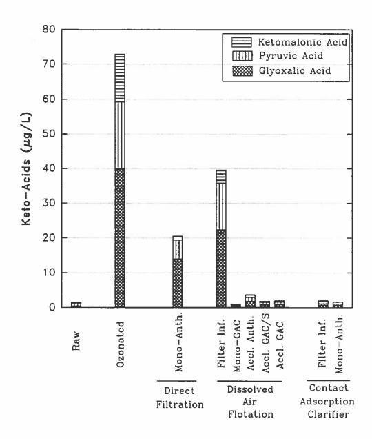
Figure 3. Keto-acids at Various Stages of Treatment on August 4, 1992. (All are filter effluents unless otherwise indicated; Mono-GAC=fresh mono-media GAC filter with F300; Accl. Anth.=acclimated mono-media anthracite filter; Accl. GAC/S=acclimated GAC/Sand dual-media with F300; Accl. GAC=acclimated GAC mono-media filter with Nuchar B)
