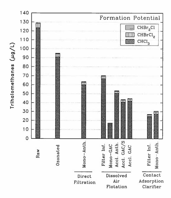
Figure 4. Trihalomethane Formation Potential at Various Stages of Treatment on August 4, 1992. (All are filter effluents unless otherwise indicated; Mono-GAC=fresh monomedia GAC filter with F300; Accl. Anth.=acclimated mono-media anthracite filter; Accl. GAC/S=acclimated GAC/Sand dual-media with F300; Accl. GAC=acclimated GAC mono-media filter with Nuchar B)
