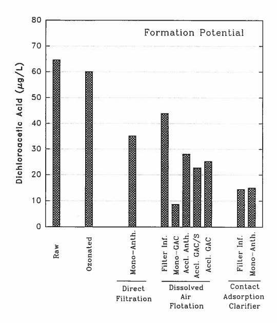
Figure 6. Dichloroacetic Acid Formation Potential at Various Stages of Treatment on August 4, 1992. (All are filter effluents unless otherwise indicated; Mono-GAC=fresh monomedia GAC filter with F300; Accl. Anth.=acclimated mono-media anthracite filter; Accl. GAC/S=acclimated GAC/Sand dual-media with F300; Accl. GAC=acclimated GAC mono-media filter with Nuchar B)
