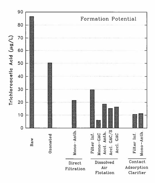
Figure 5. Trichloroacetic Acid Formation Potential at Various Stages of Treatment on August 4, 1992. (All are filter effluents unless otherwise indicated; Mono-GAC=fresh monomedia GAC filter with F300; Accl. Anth.=acclimated mono-media anthracite filter; Accl. GAC/S=acclimated GAC/Sand dual-media with F300; Accl. GAC=acclimated GAC mono-media filter with Nuchar B)
