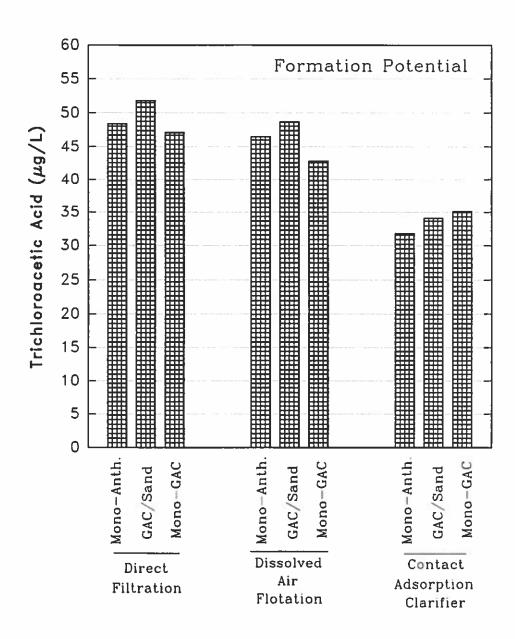
Figure 11. Trichloroacetic Acid Formation Potential in the Effluents of the Three Acclimated Filters for the Period February 17-20, 1992. (Mono-Anth.=mono-media anthracite filter; GAC/Sand=dual-media filter with F300 and sand; Mono-GAC=mono-media filter with Nuchar B)
