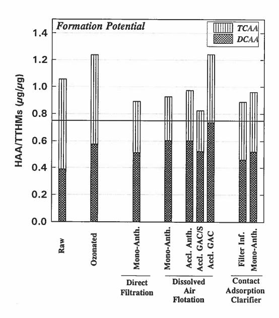
Figure 14. Haloacid to Trihalomethane Formation Potential Ratios at Various Stages of Treatment on May 14, 1992. (All are filter effluents unless otherwise indicated; Accl=acclimated; GAC/S=dual media filter with F300 and sand; GAC=mono-media filter with Nuchar B)
