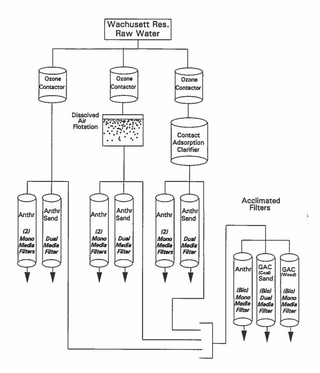
Figure 1. Process Schematic for the Wachusett Reservoir Pilot Plant
