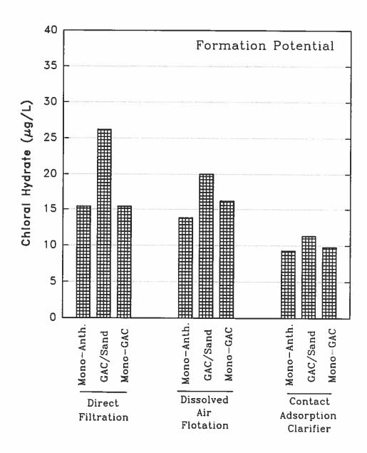
Figure 10. Chloral Hydrate Formation Potential in the Effluents of the Three Acclimated Filters for the Period February 17-20, 1992. (Mono-Anth.=mono-media anthracite filter; GAC/Sand=dual-media filter with F300 and sand; Mono-GAC=mono-media filter with Nuchar B)
